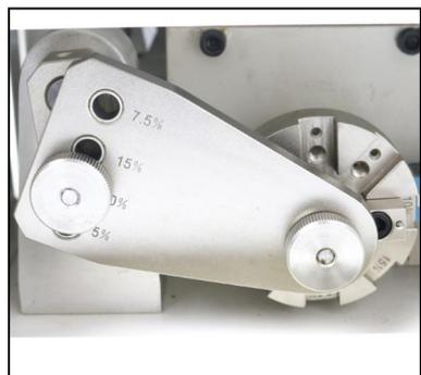
Adjust the displacement of flexing.
